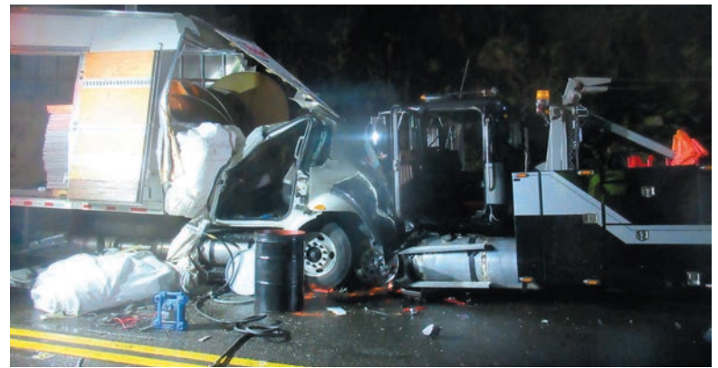
Only the steel frame of the tow truck kept the rental truck from smashing into the windshield.
